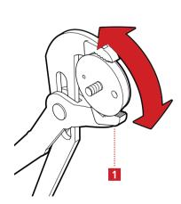
1 Adapter entfernen Remove adapter w/ pipe wrench
